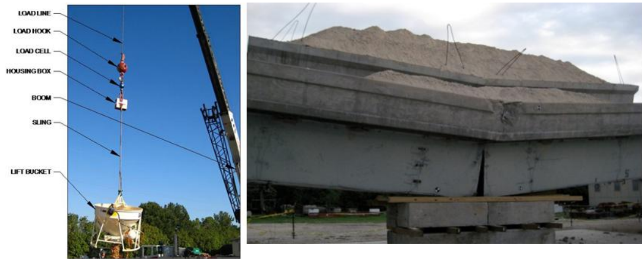
Figure 9. Bridge collapse test crane load measurements.
