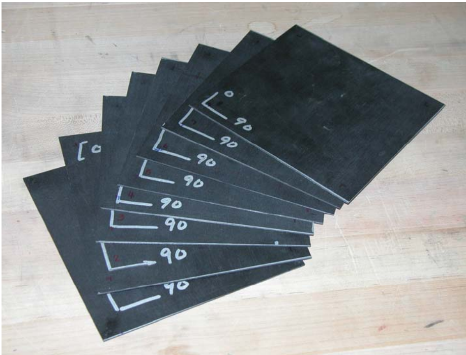
Figure 1. Population of eight nominally identical laminated composite plates.
